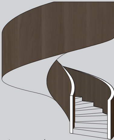
Rivestimento scale curve. Curved staircase covering.
